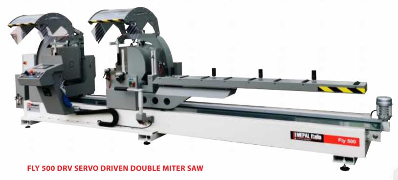
The FLY 500 DRV Double Miter Saw is a servo length positioned, double miter back cut saw with a fixed left head and numerically controlled positioning right head. Cut angles can be set by pneumatic actuators from 45°/90°/135° and intermediate angles utilize a manual set stop. The machine is equipped with a V8 touchscreen industrial CNC for easy operator interface.
